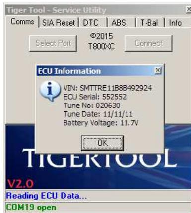
If the ECU type-check matches and data was read successfully, the 'ECU Information' pop-up box should appear, as shown above, to display the VIN number, ECU serial number, engine map/tune number, the date the tune was installed, and the approximate battery voltage.
