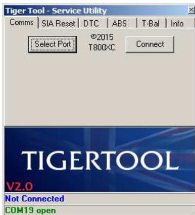
Now click the 'Connect' button to start communicating with the ELM327 interface and ECU - this may take several seconds and should indicate progress according to the following images:-
