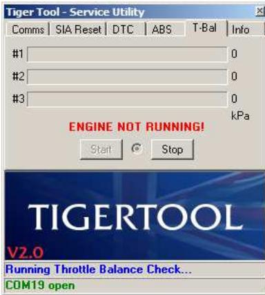
The software will continue to request the values from the ECU but as the engine is not running it should report a zero value. If you start the engine the readings should appear after a couple of seconds.
