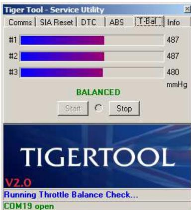
The flashing dot between the 'Start' & Stop' buttons is there to indicate that the engine is running and that readings are being taken.
