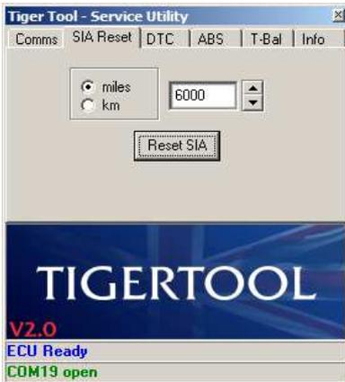
Click on the check box to select either 'miles' or 'km' to suit the current settings on your bike's instruments. Use the up/down arrows next to the units to scroll through to the service interval that you want to use. If you click between the miles & km check boxes on TigerTool a rough conversion will be made and the distance updated (rounded to the nearest 100 units), within the acceptable limits.
