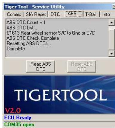
After resetting ABS DTCs it may also be necessary to re-check & reset non-ABS DTCs as some are inter-linked. You may also need to switch off the ignition, wait 1 minute then switch on again to allow the ECU and other systems to fully reset before re-checking for ABS DTCs.
