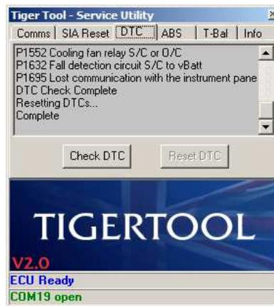
Once the DTCs have been successfully reset, you can confirm this by re-clicking the 'Check DTC' button. It may be necessary to switch off the ignition, wait 1 minute then switch on again to allow the ECU and other systems to fully reset before re-checking for DTCs.
