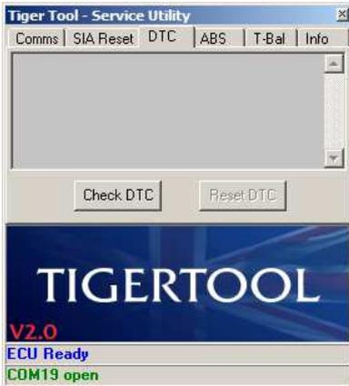
To read the list of confirmed DTCs from the ECU, click on the 'Check DTC' button and the following images should appear if no DTCs are found:-
