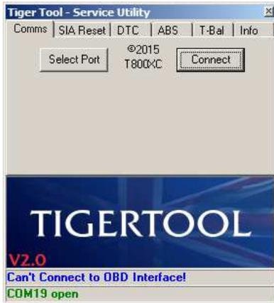
The most likely causes of this error are either the wrong serial port being selected or no power to the ELM327 interface. Try to unplug then reconnect the interface from the bike (and observe the active LEDs) and/or try a different serial port. Also make sure that the ignition & engine kill switches are on.
