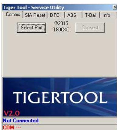
Click on the 'Select Port' button then use the arrow in the list box to select the serial port for your ELM327 interface. Depending on your PC configuration you may have several serial ports so it's worth looking at Windows Device Manager to check which one is assigned to your ELM327 interface. In the case of Bluetooth interfaces, there may be two assigned serial ports (depending on the drivers) so you may have to try both to see which one provides access.
