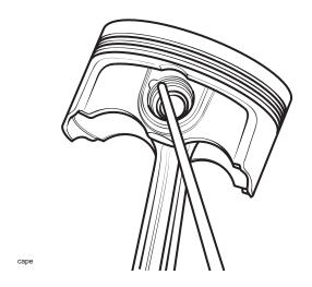
Removing the Gudgeon Pin Circlip
