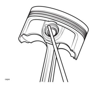
Removing the Gudgeon Pin Circlip
