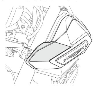
Masked Area (Left Hand Side Fairing Shown with High Level Mudguard Removed for Clarity)
